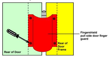
**Step 3:** Peel off the protective tape from one side of the door finger guard. Line up the edge of the door finger guard to the guideline on the door-frame and press firmly in place.
